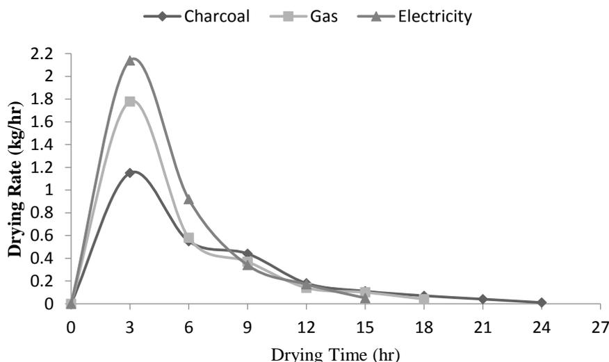
Figure 2: Drying rate curve of *C. gariepinus* smoked, dried in the three NSPRI fish kilns
