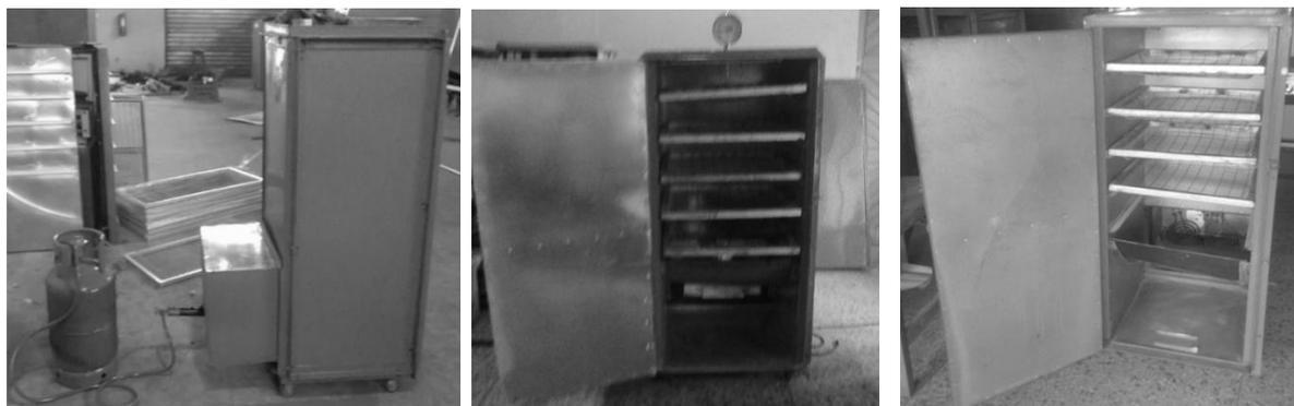
Plate 1: Gas powered fish kiln      Plate 2: Charcoal powered fish kiln      Plate 3: Electrically powered fish kiln
