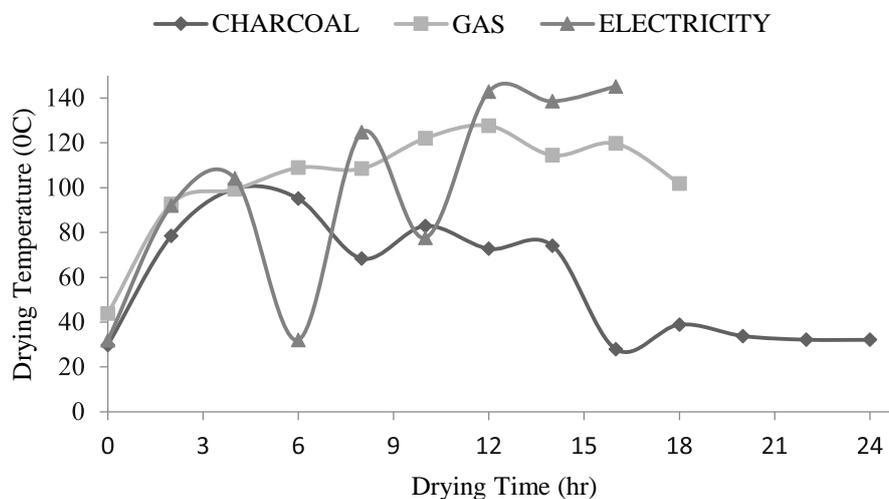
Figure 1: Temperature profiles of the NSPRI fish kilns
