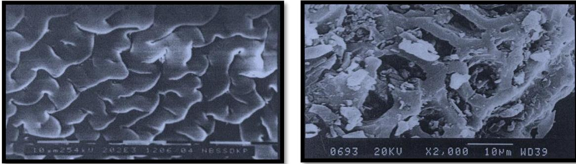
**Fig. 3.1. SEM Micrograph of Groundnut Shell before and after Activation**
